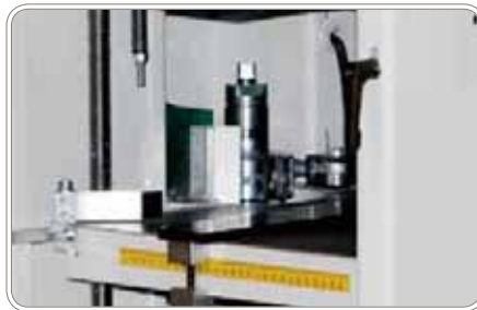
You plane the workpiece into width and height in one single operation. With the side cutter you can also mould the timber.
